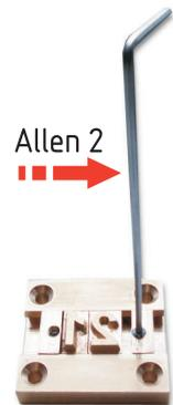
**IMPORTANT:** To replace the letters the device must be completely cooled!
